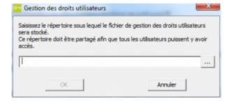
The dialog box allows you to enter this directory. If it is located on another machine (server accessible by the network, for example), it is preferable to indicate it in a relative way \\server\path\. It will contain the following elements:
