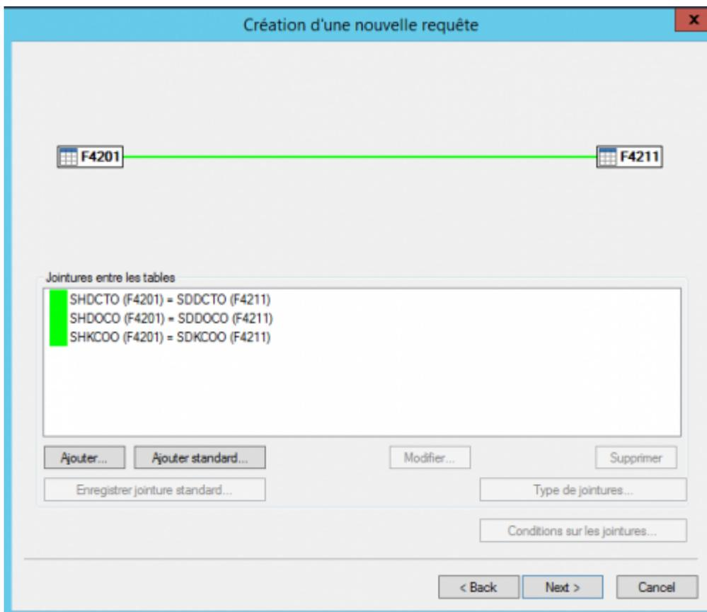
When joints have been modified or added manually, it is possible to add them to the Vigilens standard joints library: just use the button Record standard joints, a screen allows you to select the joints
