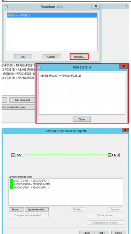
When joints have been modified or added manually, it is possible to add them to the Vigilens standard joints library: just use the button Record standard joints, a screen allows you to select the joints
