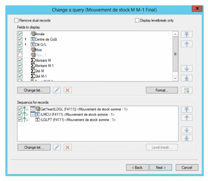
This screen displays a list of all fields displayed, whether they come from a table, a field in a subquery, or a calculated field (operation, see OPManage).
