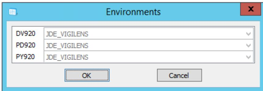
This screen lists all the parameterized environments and allows, for each of them, to specify the corresponding database. This parameterization is used for the dynamic management of query execution environments from JDE (JDEUTIL prerequisite).
